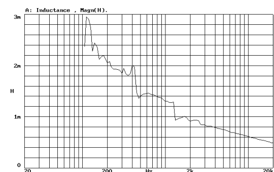
VOICE COIL INDUCTANCE CURVE
